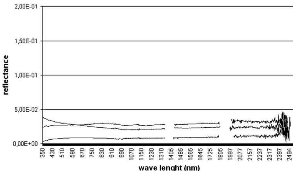
Fig. 6. Spectral signatures on three Balchit obsidian samples.
