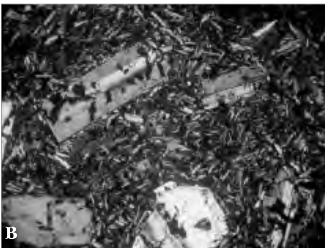
Fig. 5. Doleritic porphyric lava at Wutale East Gully: A, natural light; B, polarized light. Cliché G. Kieffer
